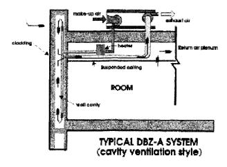
Fig 10. DBZ with ventilated cavity
