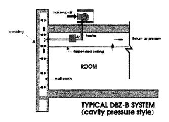
Fig 11. DBZ with pressurized cavity
