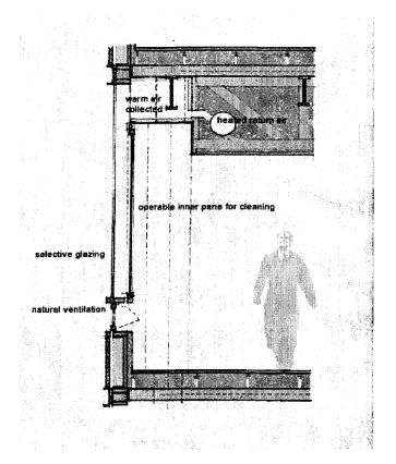
Fig 7. Wall section detail of the CDP
