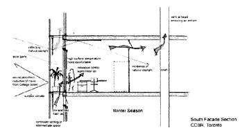
Fig 5. Winter condition of the south façade of the CCBR at University of Toronto
